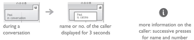
Depending on how the system is configured, the name or number of the caller is displayed on the screen. Pressing the 'i' key displays the name or number of the caller on the screen. If the number is displayed by default, pressing the 'i' key displays the name. If the name is displayed by default, pressing the 'i' key displays the number.
