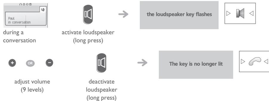
*press and release the loudspeaker key to switch to hands free mode (light steady).*
