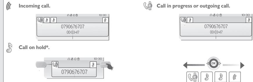
If you get two calls at the same time, you can switch from one call to the other by pressing the display key associated with each call. **Left-right navigator:** used to check calls.
