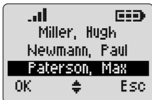
The two keys below the display, as well as the arrow keys, are known as softkeys. The functions assigned to the keys are shown in the lowest line of the display. The key function changes automatically according to the operating status of the handset.
