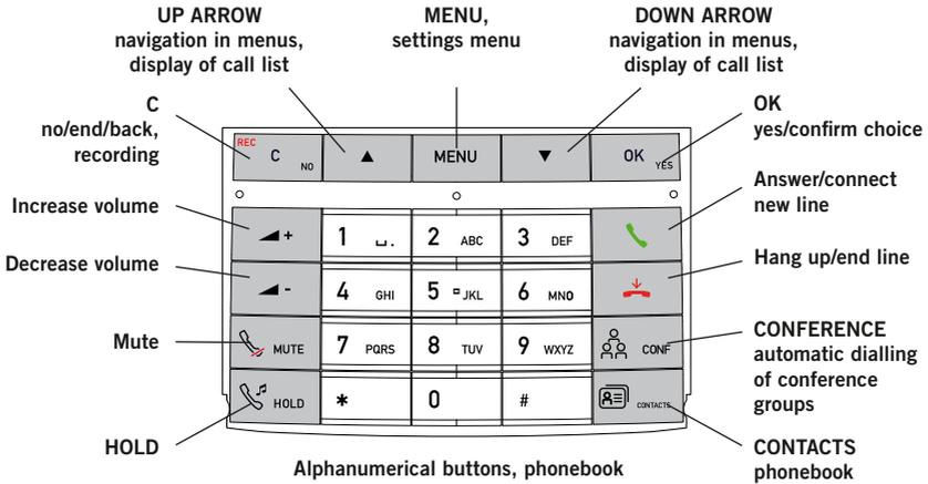
ⓘ Some OmniTouch 4135 IP have a different keypad with other symbols. This does not affect the functions of the buttons
