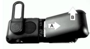
Remove the battery from its compartment as shown in the drawing.
