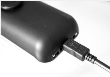
Plug the USB cable into the USB port of your phone. The other end of the USB cable can be plugged into the AC/DC adaptor or into a computer USB port.
