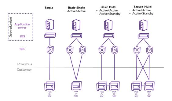
By default, the Service is activated in **Basic-Single** mode, where the IP PBX is connected to 2 different network SBCs for redundancy reason.
